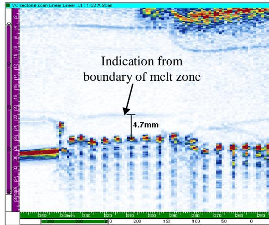
Figure 10. Ultrasonic image of a standard 450 mm (18 inch) SDR17 EF joint.
