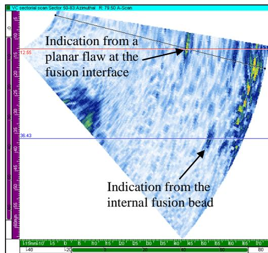
Figure 12. Ultrasonic image of a 355 mm (14 inch) SDR11 BF joint containing a 4 mm (0.16 inch) planar flaw at the fusion interface.
