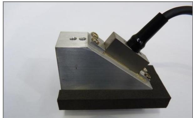
Figure 4. Angled water wedge/probe assembly used for inspecting small diameter BF joint.
