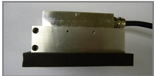
Figure 3. Zero degree water wedge/probe assembly used for inspecting small diameter EF joints.
