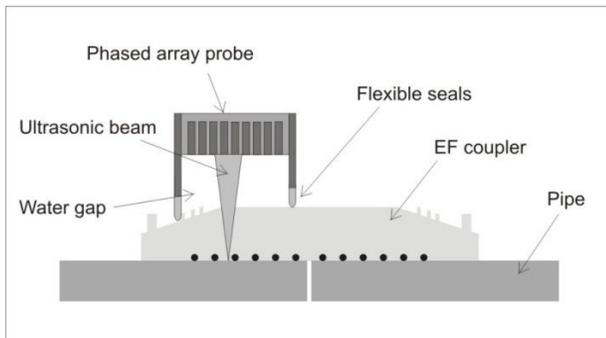
Figure 2. Inspection technique used for EF joints.
