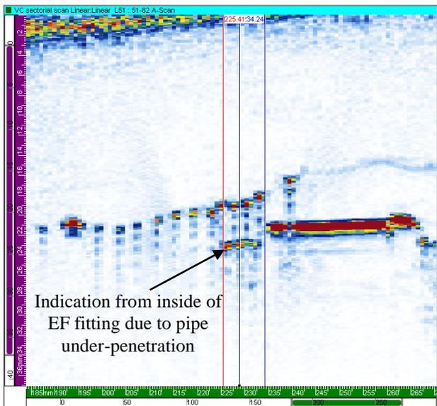
Figure 9. Ultrasonic image of a 225 mm (9 inch) SDR11 EF joint where the pipe has not been fully inserted into the coupler.
