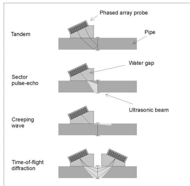
Figure 1. Inspection techniques used for BF joints.
