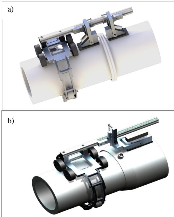
Figure 5. CAD design of the TestPEP inspection system without an encoder on the carriage for: a) BF joints, and b) EF joints.
