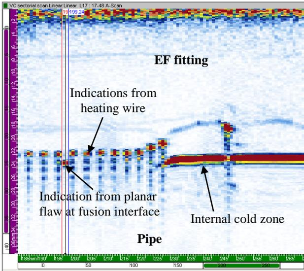
Figure 8. Ultrasonic image of a 225 mm (9 inch) SDR11 EF joint containing a 2 mm (0.08 inch) planar flaw at the fusion interface.
