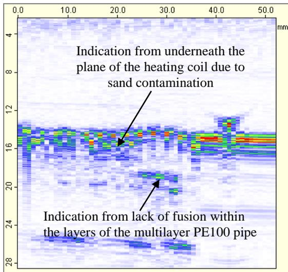
Figure 13. Ultrasonic image of an EF joint produced by E.ON Ruhrgas containing sand contamination.
