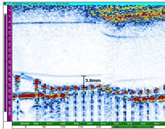
Figure 11. Ultrasonic image of a 450 mm (18 inch) SDR17 EF joint where the heating time has been reduced by 50%, resulting in a cold fusion.
