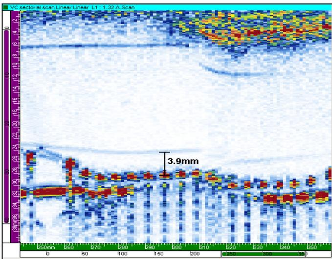
**FIG. 12 IMAGE OF AN EF JOINT IN 450MM PE PIPE WITH COLD FUSION**
