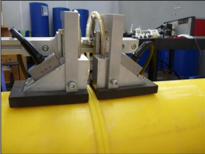
**FIG. 14 ANGLED WATER WEDGES USED FOR INSPECTING BF WELDS**
