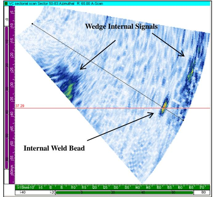
**FIG. 15 IMAGE OF A BF JOINT IN 355MM PE PIPE WITH NO FLAWS**
