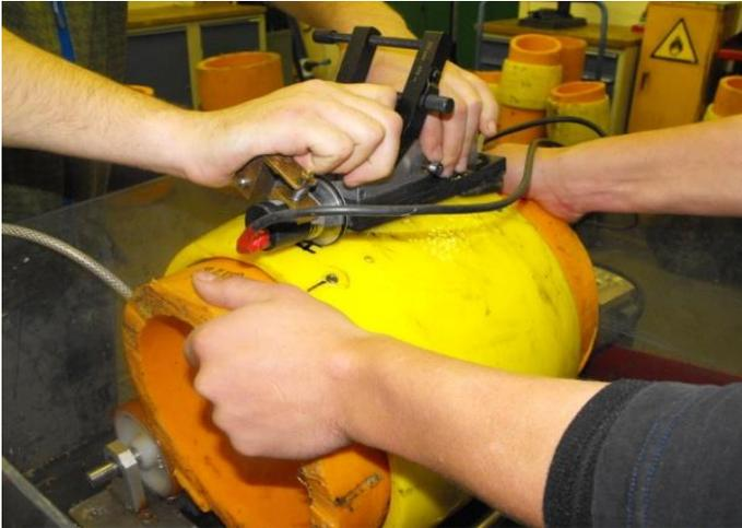
**FIG. 27 HAND MANIPULATION OF PROBE TO INSPECT CUT OUT SAMPLE EF JOINT**
