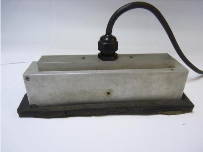
**FIG. 7 ZERO DEGREE WATER WEDGE USED FOR EF INSPECTIONS**
