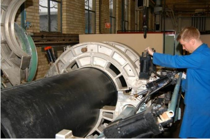
**FIG. 1 BUTT FUSION WELDING OF PE PIPES**
