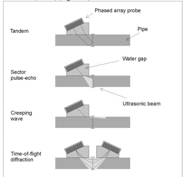
**FIG. 13 INSPECTION TECHNIQUES USED FOR INSPECTING BF WELDS**
