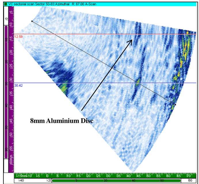
**FIG. 16 IMAGE OF A BF JOINT IN 355MM PE PIPE WITH AN 8mm ALUMINIUM DISC**
