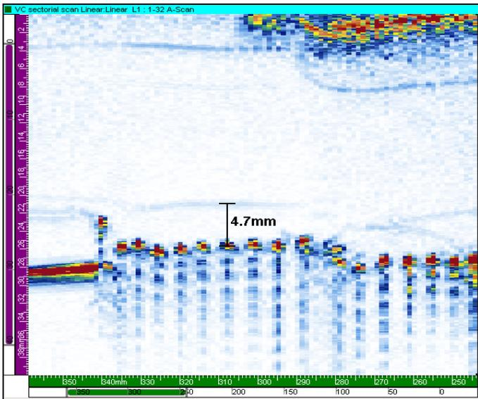
**FIG. 11 IMAGE OF AN EF JOINT IN 450MM PE PIPE WITH GOOD FUSION**
