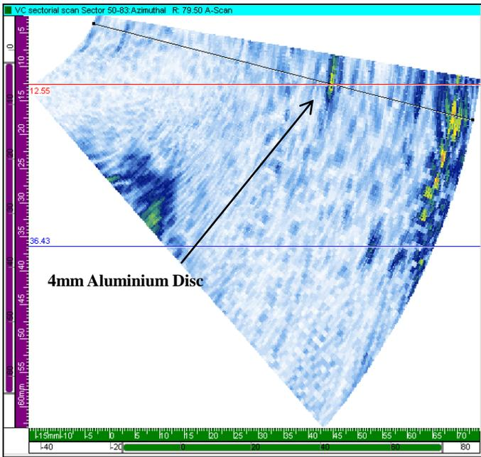
**FIG. 17 IMAGE OF A BF JOINT IN 355MM PE PIPE WITH A 4mm ALUMINIUM DISC**
