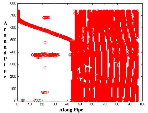
**FIG. 19 DETECTION OF THE ZONES CORRESPONDING TO THE HEATING WIRES**
