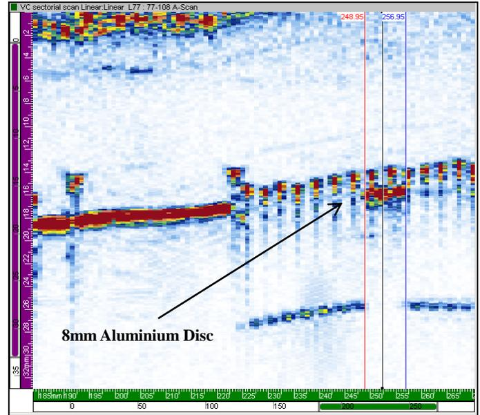
**FIG. 9 IMAGE OF AN EF JOINT IN 180MM PE PIPE WITH AN 8mm ALUMINIUM DISC**
