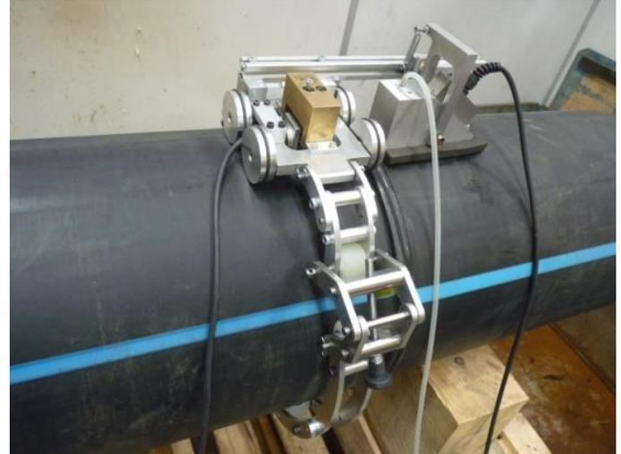
**FIG. 26 FLEXIBLE CHAIN LINK SCANNER WITH BF PROBE HOLDER**
