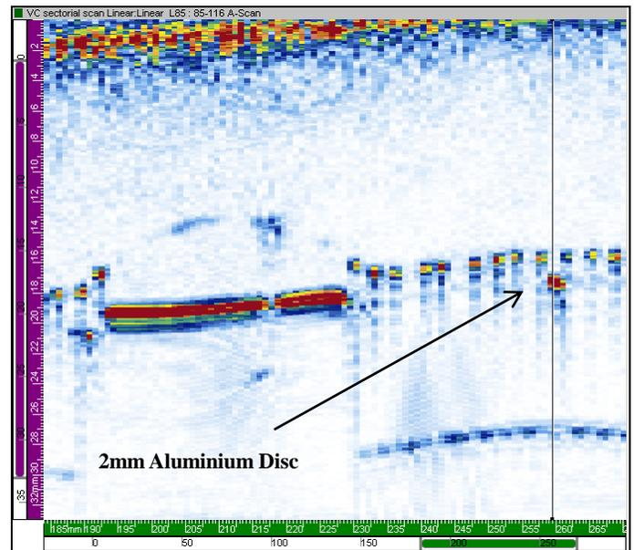
**FIG. 10 IMAGE OF AN EF JOINT IN 180MM PE PIPE WITH A 2mm ALUMINIUM DISC**
