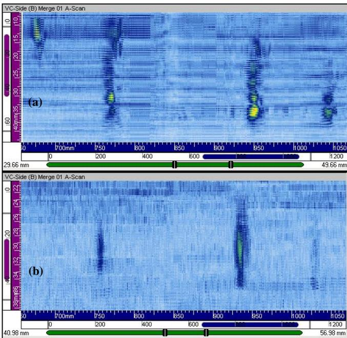
**FIG. 18 MERGED B SCAN USING (a) SECTOR PULSE ECHO (b) SELF-TANDEM**
