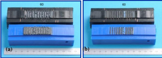
**FIG. 24 FRACTURE SURFACES OF PEEL DECOHESION TEST SPECIMENS FROM EF JOINTS IN 225MM PIPE WITH (A) DUCTILE FRACTURE THROUGH THE PLANE OF THE HEATING WIRES, AND (B) BRITTLE FRACTURE THROUGH THE WELD INTERFACE.**
