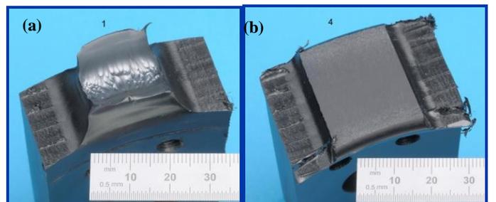
FIG. 23 FRACTURE SURFACE OF TENSILE TEST SPECIMENS FROM 225MM PE PIPE WITH (A) FULLY DUCTILE FAILURE, AND (B) FULLY BRITTLE FAILURE.
