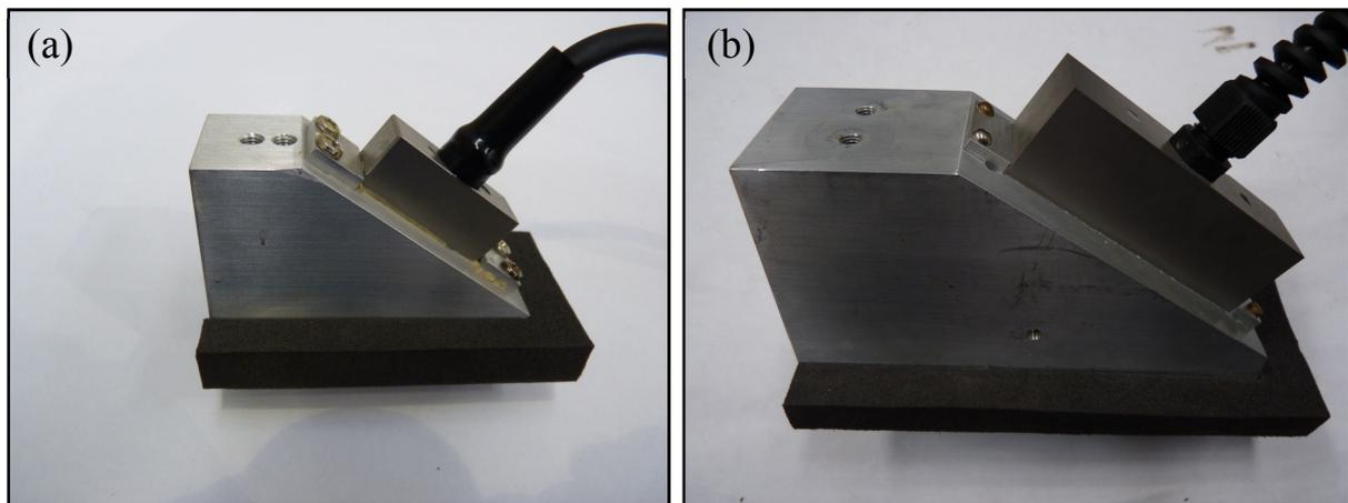
**Figure 4** Angled water probe wedges. (a) 4MHz and (b) 2MHz.
