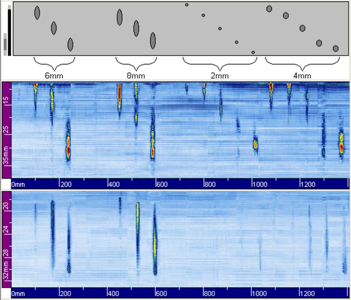
**Figure 8** Schematic drawing of the cross-section of the 450mm OD and 28mm thick pipe with FBHs and the sector pulse-echo and tandem inspection results.
