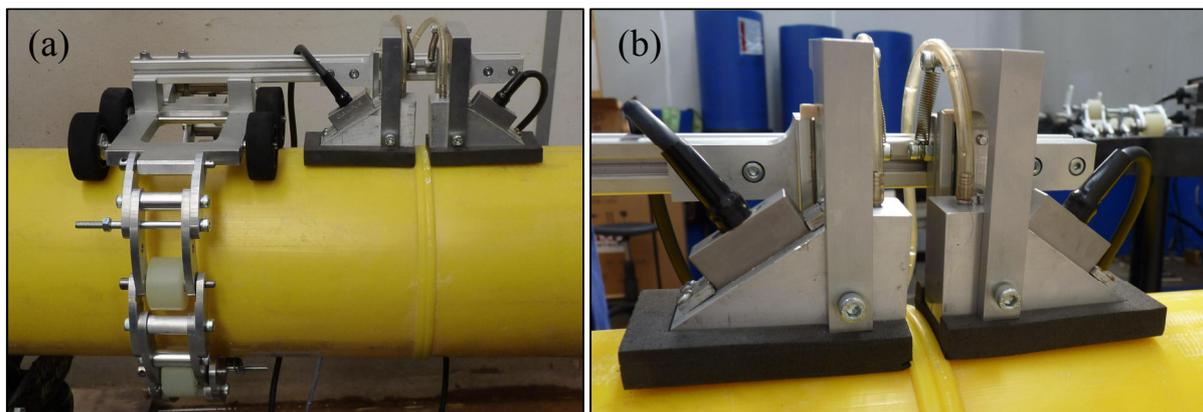
**Figure 5** (a) The flexible chain link scanner with the 4MHz probes. (b) BF probe holder.
