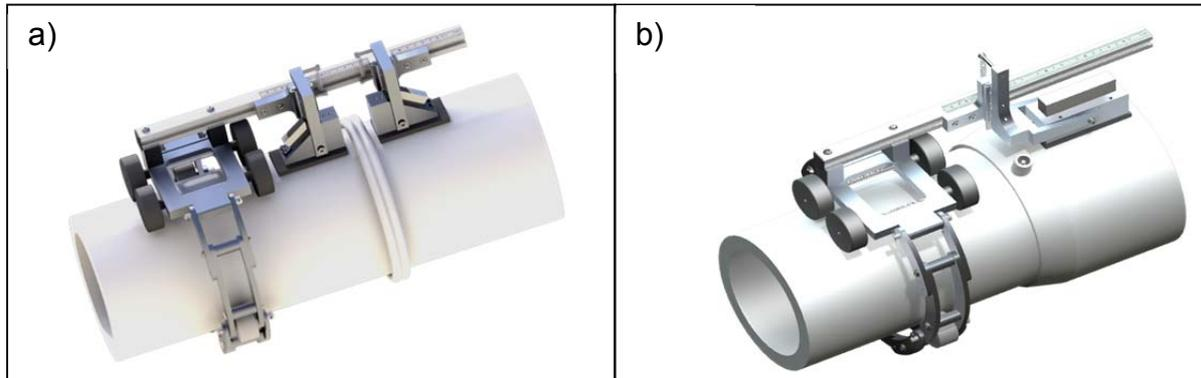
Since the aim of the project is to have the flaw detector mounted on the carriage of the scanner with wireless connection to a remote computer, a new compact phased array flaw detector with the ability to operate in a harsh environment has been designed and manufactured, with the following features:
