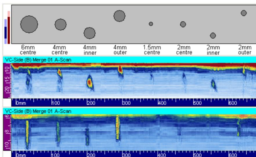
**Figure X: B-scan images from creeping wave and TOFD scans on 225mm (9 inch) diameter PE pipes containing slots**
