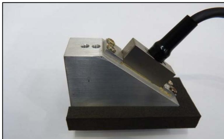
In order to develop the PAUT technique for the EF joints, initial inspection trials were carried out using unwelded EF fittings, based on the assumption that, if sufficient resolution can be achieved to detect the wires, the fusion zone located just below the wires can also be inspected.
