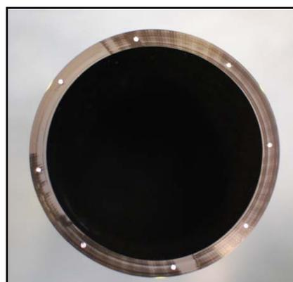
After welding, the joint was cut out and machined to a thickness equal to that of the weld beads (Figure II) before being inspected using X-ray radiography to determine the final positions of the discs after welding (Figure III).
