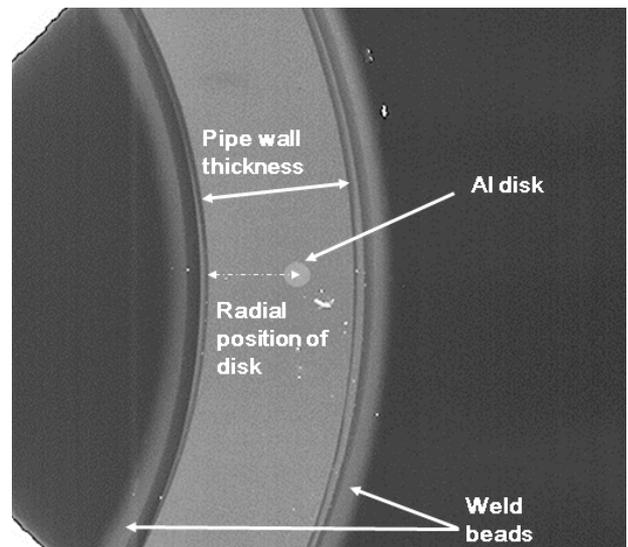
**FIG. 6 RADIOGRAPH SHOWING FINAL POSITION OF ALUMINUM DISC AFTER WELDING**
