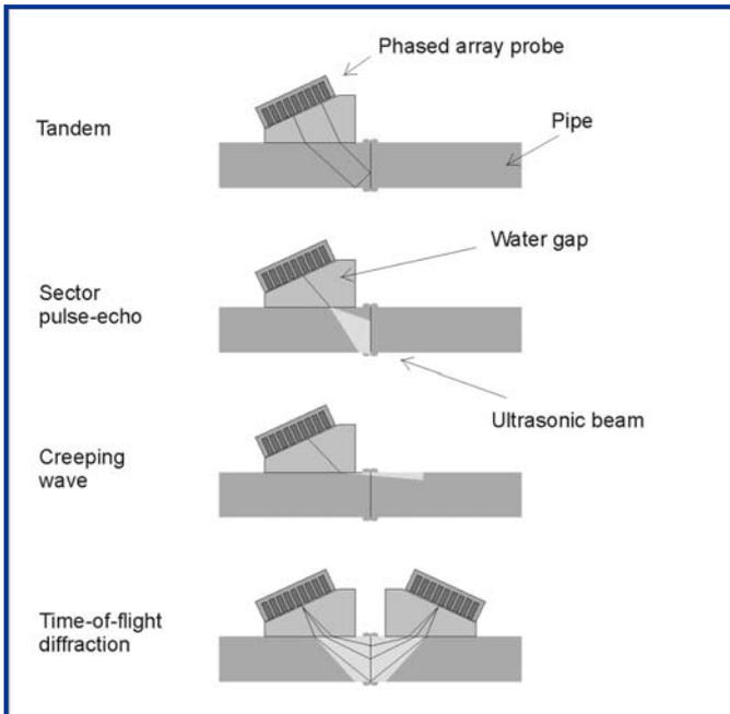
**FIG. 11 INSPECTION TECHNIQUES USED FOR INSPECTING BF WELDS**
