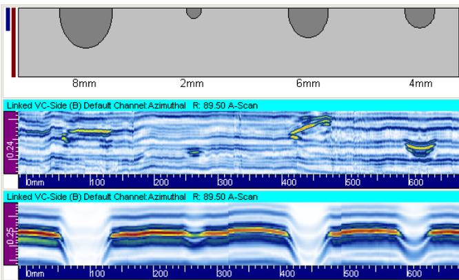
**FIG. 16 DEVELOPED VIEW OF SLOTS IN A 225MM PE PIPE USING THE CREEPING WAVE AND TOFD TECHNIQUES**
