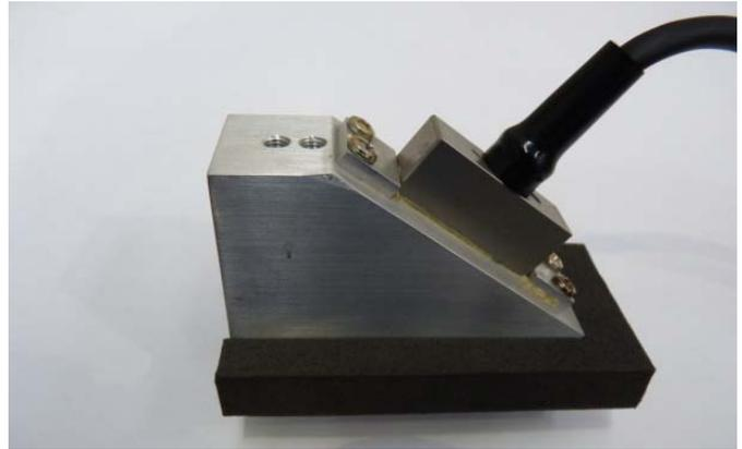
**FIG. 12 ANGLED WATER WEDGE USED FOR INSPECTING BF WELDS**
