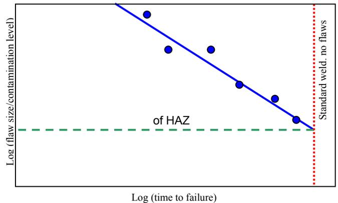
**FIG. 17 SCHEMATIC OF THE TYPE OF GRAPH USED TO DETERMINE CRITICAL DEFECT SIZES AND CONTAMINATION LEVELS**
