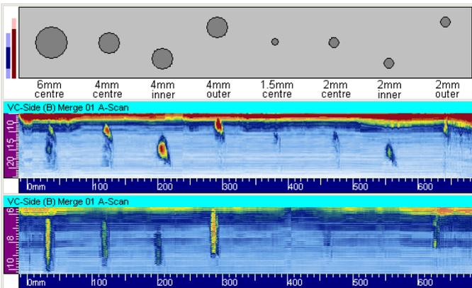
**FIG. 15 DEVELOPED VIEW OF FBHS IN THE END OF A 225MM PE PIPE USING THE SECTOR PULSE-ECHO AND TANDEM TECHNIQUES**
