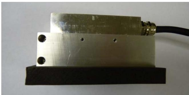
**FIG. 8 ZERO DEGREE WATER WEDGE USED FOR EF INSPECTIONS**
