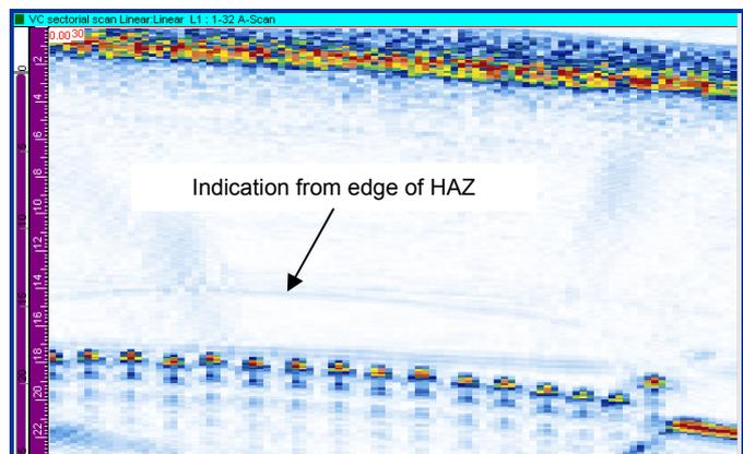
**FIG. 10 PHASED ARRAY ULTRASONIC IMAGE OF AN EF JOINT IN 180MM PE PIPE**
