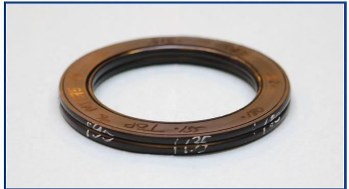
**FIG. 5 MACHINED RING OF BF WELD CONTAINING ALUMINUM DISCS**
