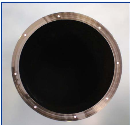
**FIG. 4 LOCATION OF ALUMINUM DISCS PRIOR TO BF WELDING**
