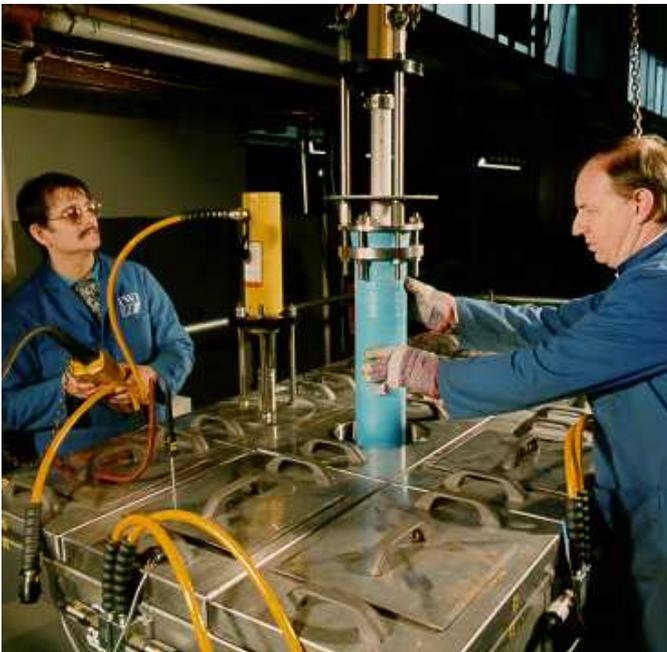
**FIG. 18 WHOLE PIPE TENSILE CREEP RUPTURE TEST RIG**
