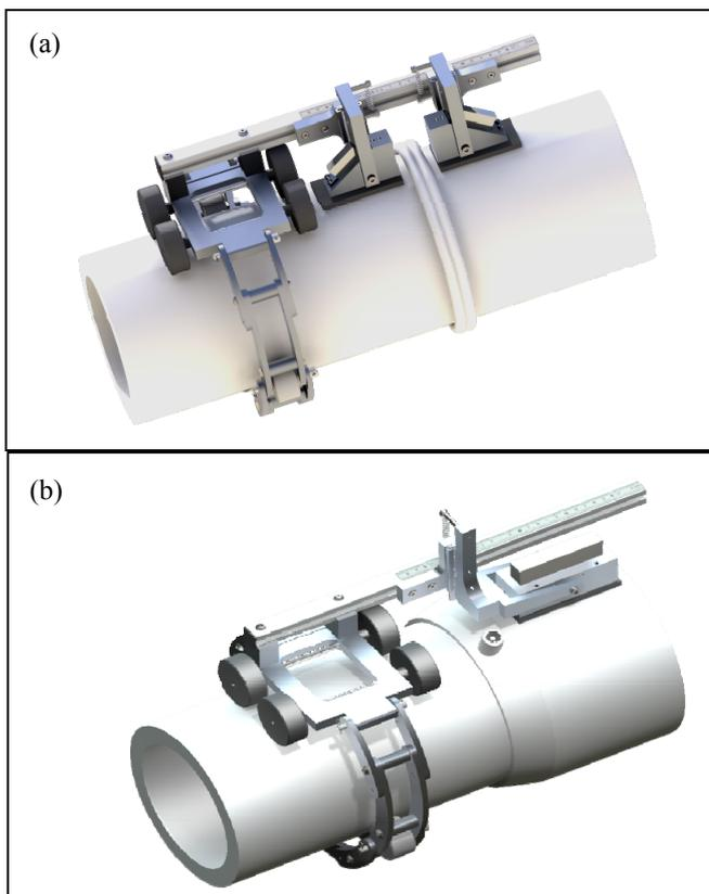
**FIG. 20 FLEXIBLE CHAIN LINK SCANNER: (a) WITH BF PROBE HOLDER, (b) WITH EF PROBE HOLDER**
