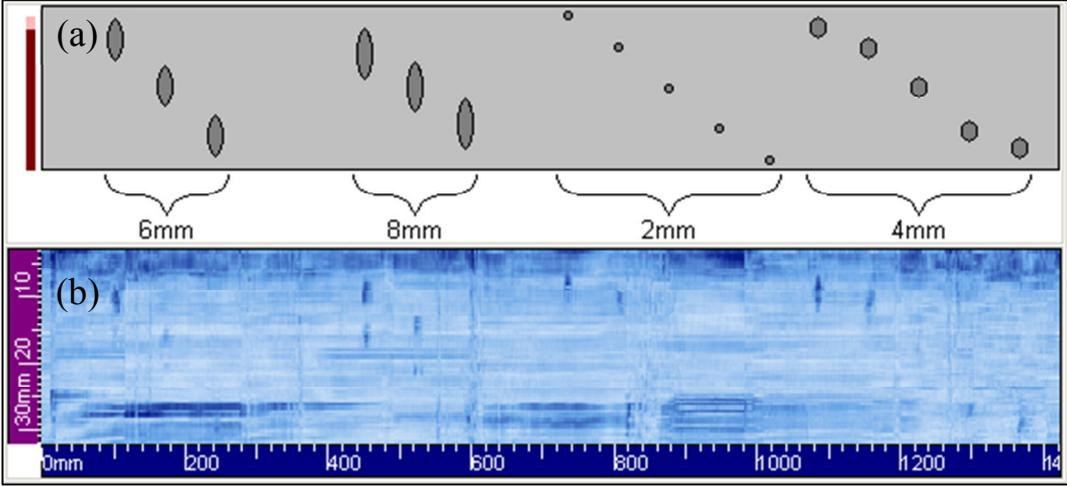
Figure 11. Inspection results on the 450mmOD pipe. (a) FBHs. (b) Sector pulse-echo scan.
