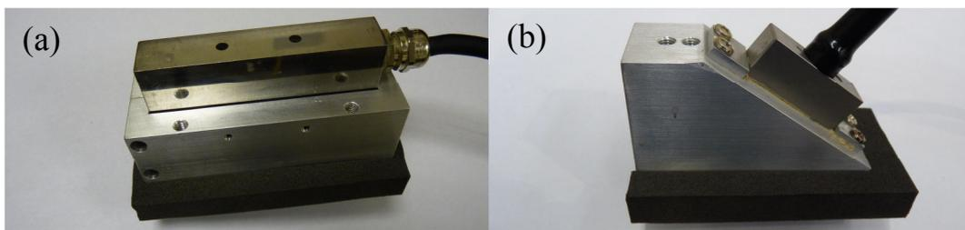
Figure 3. (a) The 0-degree water wedge. (b) The angled water wedge.
