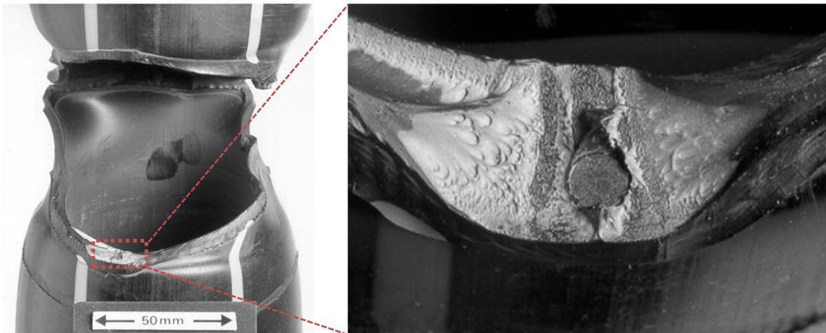
Fig. 6: Photographs of a failed weld in 125mm OD pipe containing a 4mm diameter aluminium disc.
