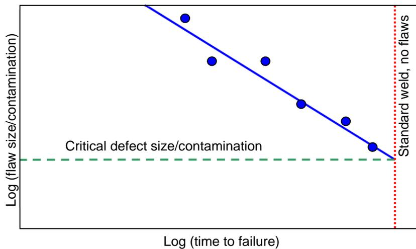
Fig. 7: Schematic of the type of graph produced to determine critical defect sizes and contamination levels.
