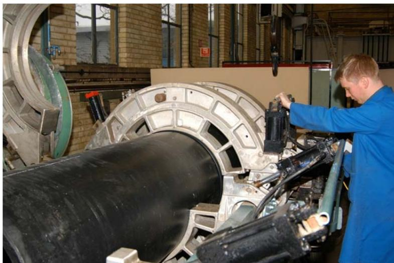
Fig.1: Butt fusion welding of PE pipes.
