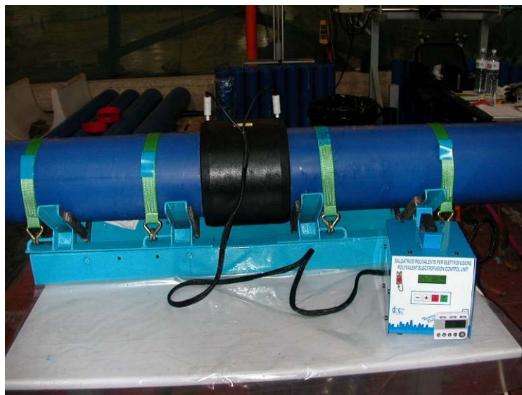
Figure 1. Electrofusion equipment and weld production
