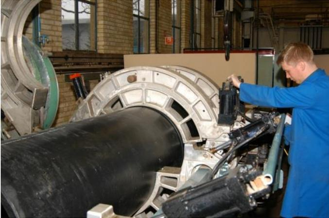
**FIG. 1 SOUDAGE BOUT A BOUT TUYAUX PE**
