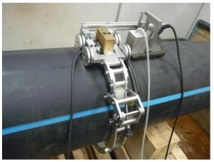
Figure 6. TestPEP inspection prototype system on a BF joint, with the encoder mounted on the carriage.
