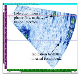
Figure 12. Ultrasonic image of a 355 mm (14 inch) SDR11 BF joint containing a 4 mm (0.16 inch) planar flaw at the fusion interface.
