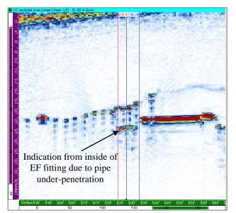
Figure 9. Ultrasonic image of a 225 mm (9 inch) SDR11 EF joint where the pipe has not been fully inserted into the coupler.
