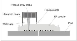
Figure 2. Inspection technique used for EF joints.
