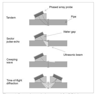
Figure 1. Inspection techniques used for BF joints.
