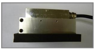
Figure 3. Zero degree water wedge/probe assembly used for inspecting small diameter EF joints.
