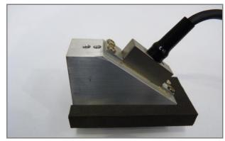
Figure 4. Angled water wedge/probe assembly used for inspecting small diameter BF joint.
