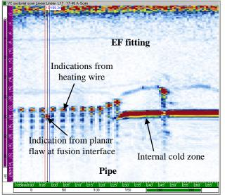
Figure 8. Ultrasonic image of a 225 mm (9 inch) SDR11 EF joint containing a 2 mm (0.08 inch) planar flaw at the fusion interface.
