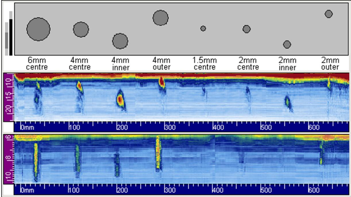
**Figure 7** Schematic drawing of the cross-section of the 220mm OD and 14mm thick pipe with FBHs and the sector pulse-echo and tandem inspection results.
