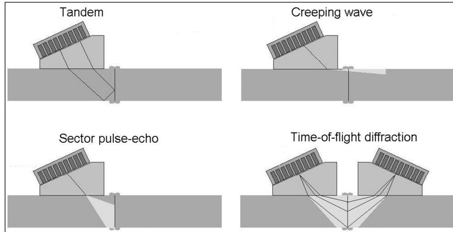
**Figure 6** Schematic drawings of the developed inspection techniques for BF joints.
