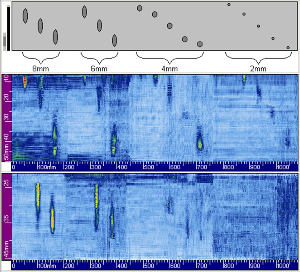
**Figure 10** Schematic drawing of the cross-section of the 710mm OD and 45mm thick pipe with FBHs and the sector pulse-echo and tandem inspection results.
