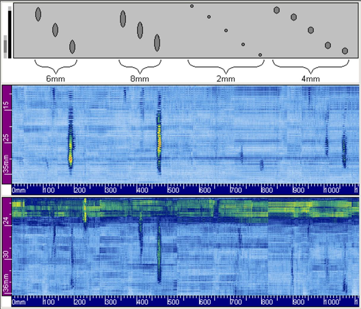
**Figure 9** Schematic drawing of the cross-section of the 355mm OD and 33mm thick pipe with FBHs and the sector pulse-echo and tandem inspection results.
