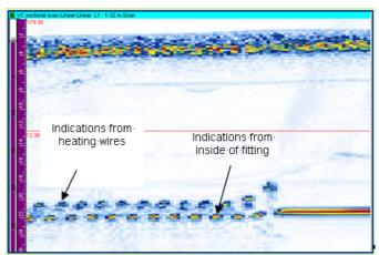
FIG. 9 PHASED ARRAY ULTRASONIC IMAGE OF 180MM EF FITTING
