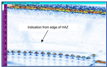
FIG. 10 PHASED ARRAY ULTRASONIC IMAGE OF AN EF JOINT IN 180MM PE PIPE
