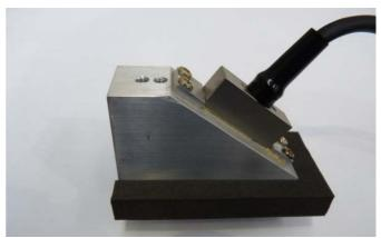
FIG. 12 ANGLED WATER WEDGE USED FOR INSPECTING BF WELDS
