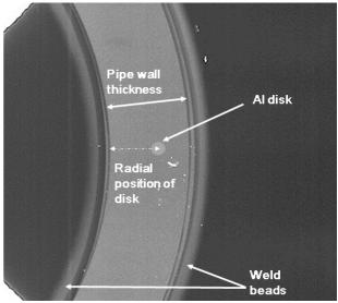
FIG. 6 RADIOGRAPH SHOWING FINAL POSITION OF ALUMINUM DISC AFTER WELDING
