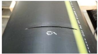
FIG. 14 SLOTS IN PE PIPE
