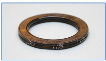
FIG. 5 MACHINED RING OF BF WELD CONTAINING ALUMINUM DISCS
