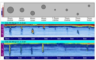
FIG. 15 DEVELOPED VIEW OF FBHS IN THE END OF A 225MM PE PIPE USING THE SECTOR PULSE-ECHO AND TANDEM TECHNIQUES
