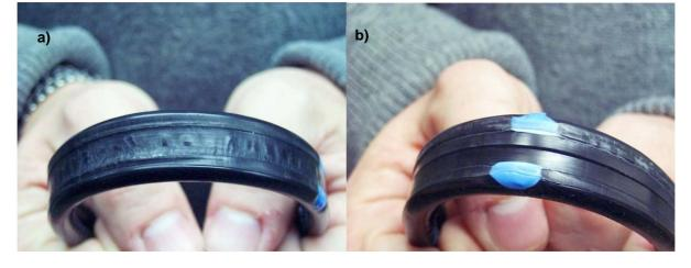
Fig. 4: Bend-back test on the external bead from welds in 315mm OD PE pipe a) containing no particulate contamination and b) containing 6% talc contamination.
