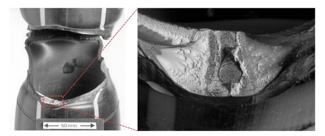
Fig. 6: Photographs of a failed weld in 125mm OD pipe containing a 4mm diameter aluminium disc.
