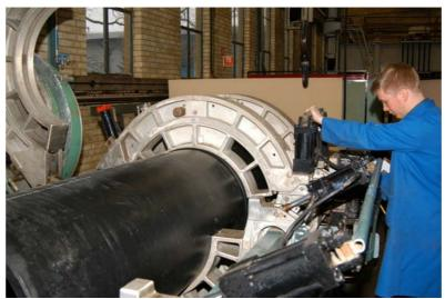
Fig.1: Butt fusion welding of PE pipes.
