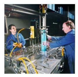
Fig. 5: Whole pipe tensile creep rupture test rig.
